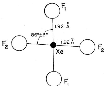
Fig. 1. The structure of the  $\text{XeF}_4$  molecule in the solid.
