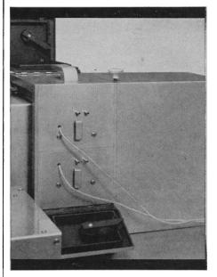
Highly versatile as a basic analytical instrument, the Perkin-Elmer Model 350 UV-VIS-NIR Spectrophotometer has even more impressive capabilities with accessories to perform extra functions. Here are some of the auxiliaries that are available: **Controlled-Temperature Cell Mount** (illustrated), for Perkin-Elmer Cylindrical Sample Cells, maintains any specified temperature from 0°C to 100°C within 0.5°C. Helps determine the kinetics of reactions at various temperatures.
