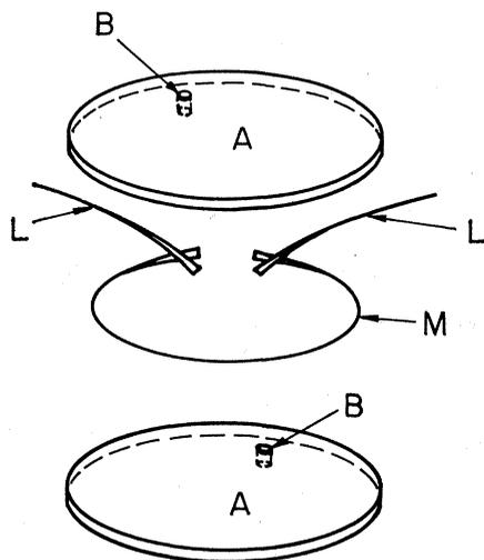
Fig. 1. Schematic sketch of setup with leads through gasket.
