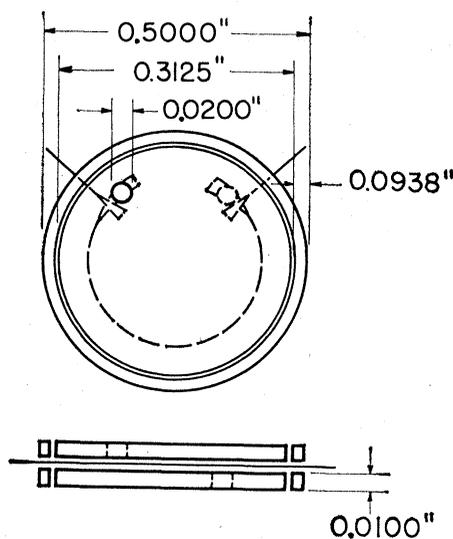
Fig. 2. Top and side views of assembly for multilead measurements.
