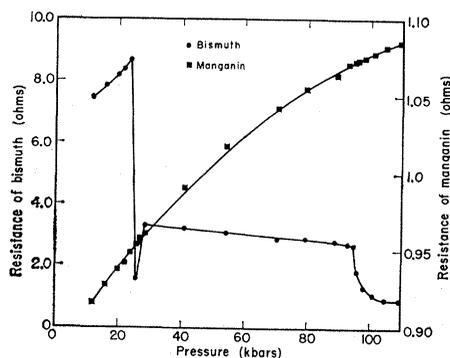
Fig. 3. Resistances of bismuth and manganin as determined simultaneously and independently with four-lead measurements.
