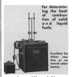
Any of seven different PARR oxygen bombs can be used in the Series 1200 adiabatic calorimeter for testing samples liberating up to 10,000 calories. The circulating water jacket surrounding the calorimeter chamber can be maintained under either adiabatic or isothermal temperature control by manual adjustment or using the new PARR 2601 Automatic Controller.
