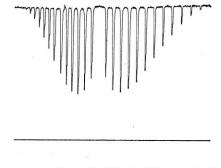
Polystyrene film. Note excellent resolution at fast scan, absence of stray light, 100% line stability, and absence of filter spikes.
