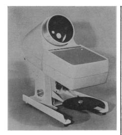
sit in a relaxed position and work in full daylight. The long eye relief (12 inches) permits the worker to wear eye glasses while using the instrument. A three-lens turret has  $7\times$ ,  $15\times$ , and  $30\times$  objective lenses. The stereomicroscope is available either with a stand or in a bench-mount version.—R.L.B. (Technitron, Inc., 2444 Wilshire Blvd., Santa Monica, Calif.)
