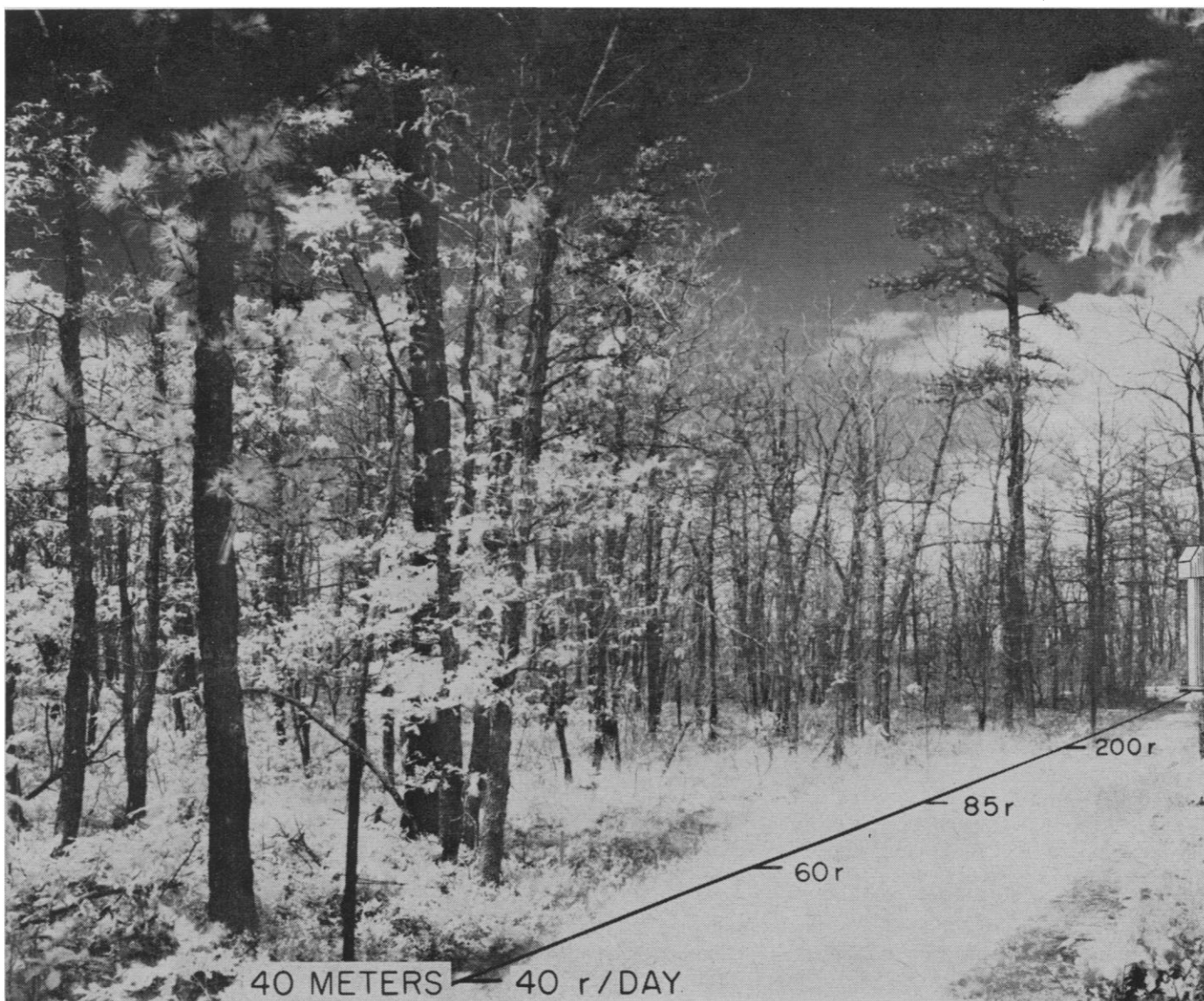
Fig. 2. The forest within 40 meters of the source after 6 months' exposure to ionizing radiation. The source is cesium-137 (9500 curies), suspended in the tower at right. The numbers indicate approximate daily exposure in roentgens, at the point indicated.
