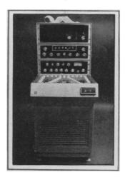
The 722 and 723 are the only commercially available room temperature, automatic liquid scintillation systems. They offer 50 sample capacity, selective sample programming, and three channel operation.
