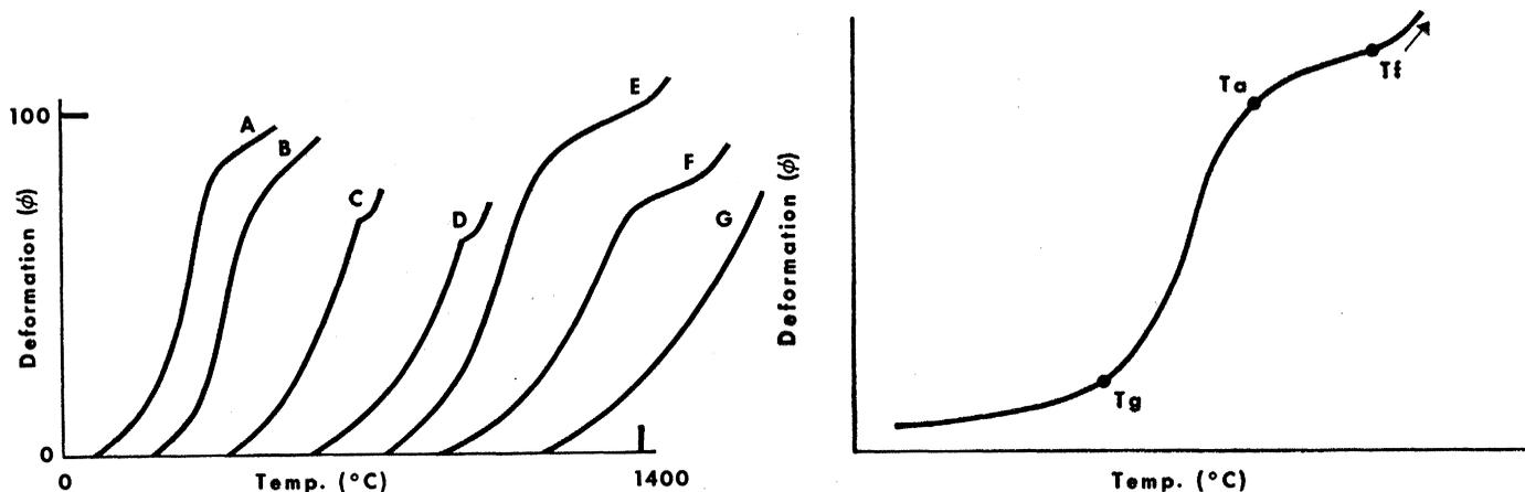
Fig. 7 (left). Deformation-temperature relationships for various glasses as follows: (A) TF-5; (B) TF-1; (C) window glass; (D) TK-10; (E) glaze; (F) glaze; (G) fused silica. Fig. 8 (right). Deformation plotted against temperature.
