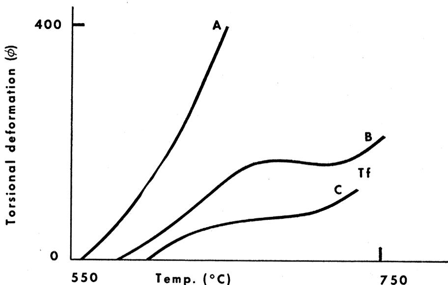
Fig. 1. Torsional deformation-temperature curves for specimens of rolled glass under various loads: (A) 93.4 g; (B) 13.2 g; (C) 11.7 g.
