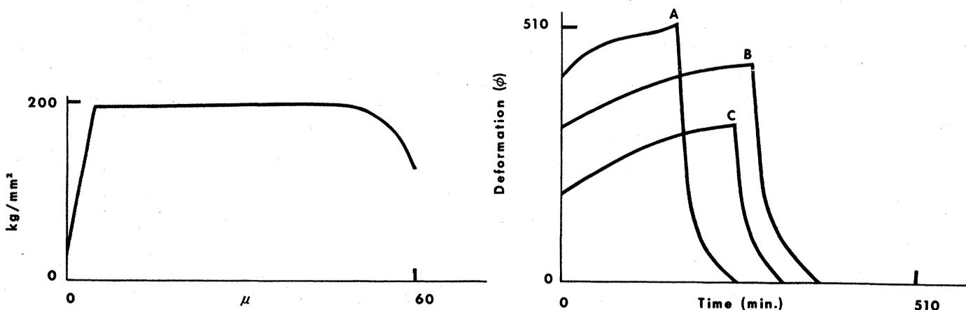
Fig. 5 (left). Effect of the thickness of the surface layer removed by etching on the strength of aluminosilicate glass fibers (diameter,  $63 \mu$ ). Fig. 6 (right). Deformation plotted against time. (A) Kerosene medium; (B) water medium; (C) potassium oleate solution.
