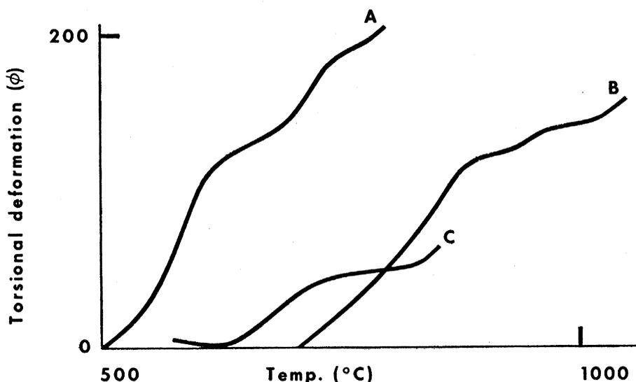
Fig. 2. Torsional deformation-temperature curves at constant torque for glasses of microheterogeneous structure. (A) Optical F-1 glass; (B) borosilicate glass; (C) high-zirconia T<sub>8</sub>-18 glass.
