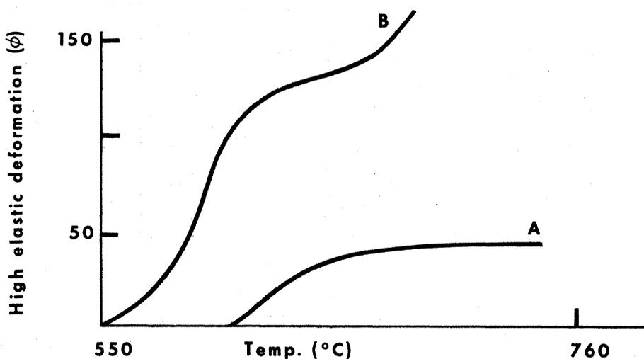
Fig. 4. Effect of heat treatment on high-elastic deformation of rolled glass. (A) Annealed specimen; (B) chilled specimen.
