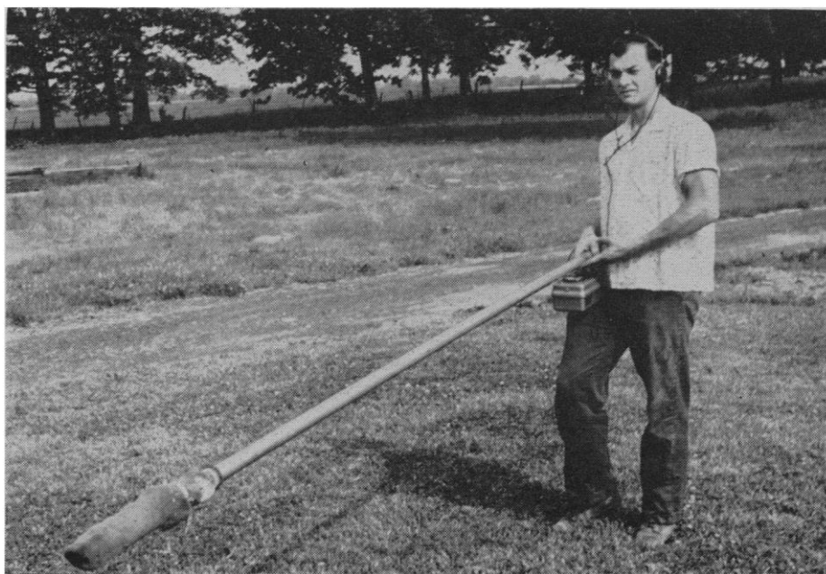
Fig. 1. The instrument used to track I^{131} -tagged Microtus pennsylvanicus in the field.
