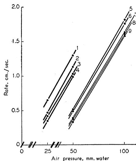
Fig. 2. Flow lines for water and eight aqueous solutions of surface active agents, all at 1 g/l: 1, water; 2, hexyl resorcinol; 3, nonyl phenol 20 EO; 4, Aerosol OT; 5, dinonyl phenol 20 EO; 6, Tween 80; 7, sodium oleate; 8, ammonium oleate; 9, Triton A-20.
