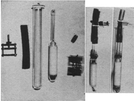
Fig. 1 (left). Materials for the ultrafiltration apparatus. (Left to right) Clamp, vacuum tubing, test tube, fritted immersion filter, grommet, dialysis tubing, and rubber band. Fig. 2 (right). Ultrafiltration apparatus (left) assembled, showing how the rubber band is used to seal the dialysis bag to the grommet, and (right) complete with close-fitting test tube; 2 ml fills the tube to the level of the grommet.
