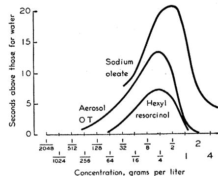
Fig. 3. Maxima in "true" meniscal resistance. Concentrations in grams per liter at which maxima occur. Time in seconds above those required for water alone (7.8 sec). Temperature, 37°C; capillary, 0.25 mm; pressure, 50 mm of water.
