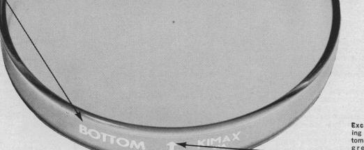
Exclusive indexing arrow on bottoms eliminates grease pencil markings.
