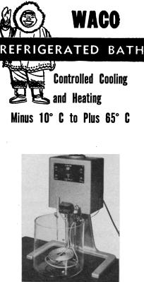
• WIDE RANGE Visibility bath with BOTH mechanical refrigeration and heating. Provides constant temperature from minus 10° C to plus 65° C using 10″ of liquid in a 16″ uninsulated Pyrex jar. Using less liquid minus 20° C is obtainable.
