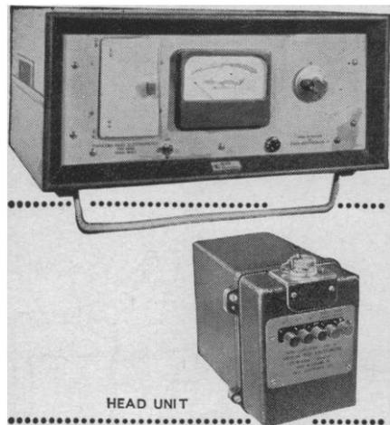
The newest Vibrating Reed Electrometer Type N616B measures direct currents down to  $-10^{15}$  amps full scale using internal resistance! Very low noise and drift— $\pm 100$  Microvolts over 24 hours. Applied D.C. is converted to A.C. by a vibrating reed capacitor and amplified by a stable A.C. amplifier. Output meter calibrated in voltage plus recorder output facility. Proven performance at low cost!
