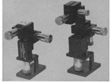
These units are designed to afford the maximum flexibility in the minimum space. Two models are available. CS-56-3 has  $\frac{5}{8}$  inch linear movement in the X,Y,Z planes. CS-56-4 has both linear and angular movement (X-25°-0-35° and Y-15°-0-15°). All linear dials are graduated in thousands of an inch.
