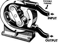
Fluids flow through a flexible tube without contacting the pump. CAPACITIES UP TO 185 G.P.H.
