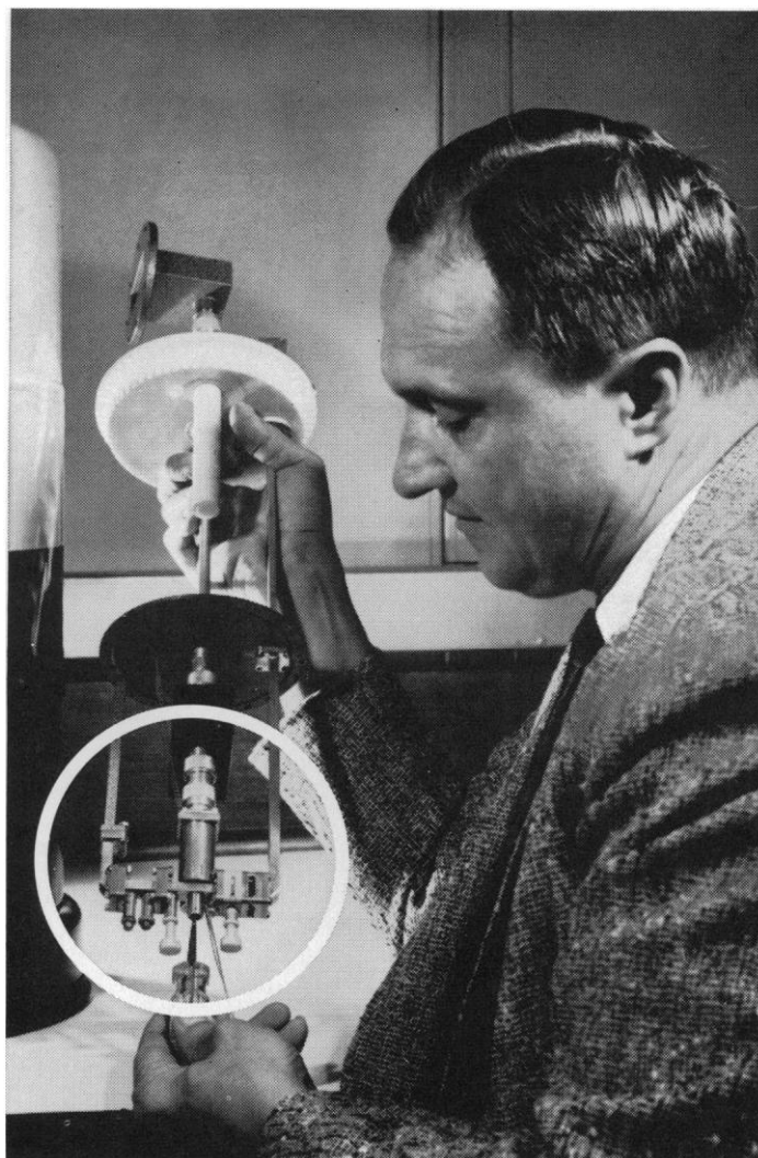
Bell Laboratories' Michael Chrunev adjusts waveguide assembly (in circle) housing the diode. After adjustment the entire parametric amplifier will be immersed in liquid nitrogen in dewar at left. The new amplifier operates at 4170 megacycles (center of band) and provides an almost flat gain of 38 db over a 50-megacycle band with a noise figure of approximately 0.6 db.
