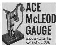
The most convenient and economical instrument for measuring low pressures from 1 micron up. Ace McLeod Gauge, supplied with Hammertone green stand, has metal locking device with position holding action eliminating the need for glass hooks and springs, will hold to any position to which it is rotated. Calibrated TRUBORE® Tubing assures accuracy and changeability in each of the following pressure ranges:
