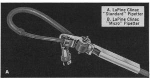
LaPine Clinac Pipetters provide complete safety from all types of contamination by eliminating mouth pipetting. They give superb, precise control with a simple, easy-to-use thumb roller.
