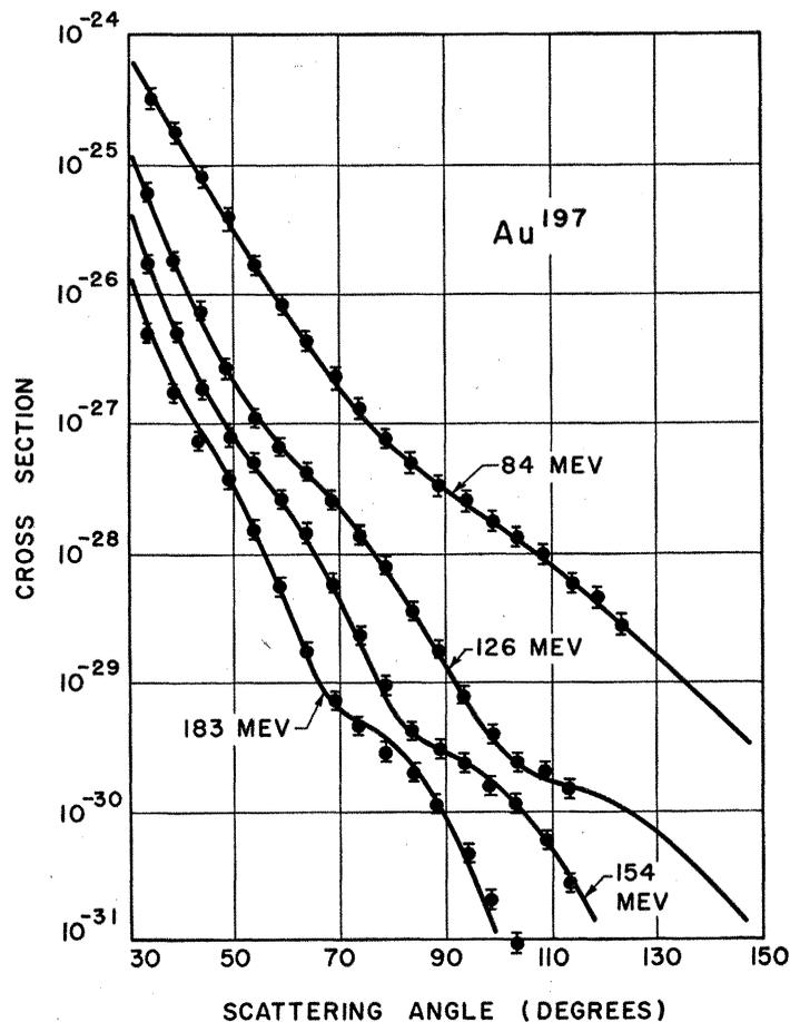
Fig. 7. The points represent experimental data observed by scattering electrons of the appropriate incident energies from gold nuclei (9). The solid lines are calculated angular distributions for a model of the gold nucleus similar to the model shown in Fig. 6.
