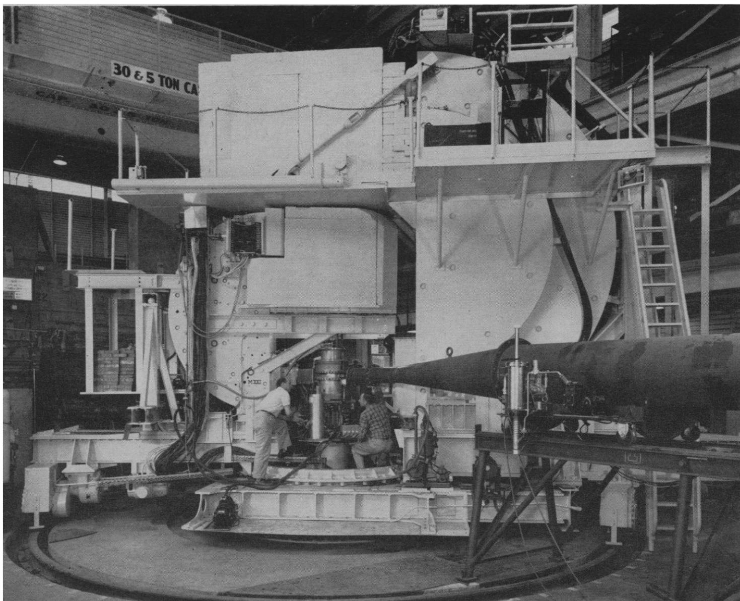
Fig. 3. A recent photograph of the double spectrometer system. The shield of the smaller spectrometer can be removed easily with the aid of an auxiliary stand. The long tube in the foreground is the vacuum pipe leading to the Faraday cup. The auxiliary stand and the Faraday cup are not shown.
