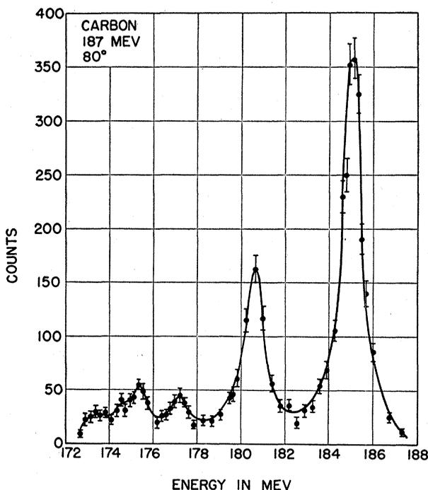
Fig. 4 (above). The elastic-scattering peak from carbon at an abscissa near 185 Mev and the inelastic-scattering peaks from the excited states of  $C^{12}$ . The peak near 180.7 Mev is associated with the 4.43-Mev level. [From J. H. Fregeau and R. Hofstadter (8)]
