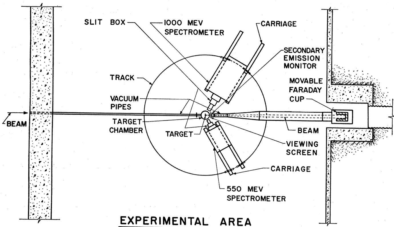
Fig. 2. Schematic diagram of a modern electron-scattering experimental area. The track on which the spectrometers roll has a radius of approximately 13.5 feet.
