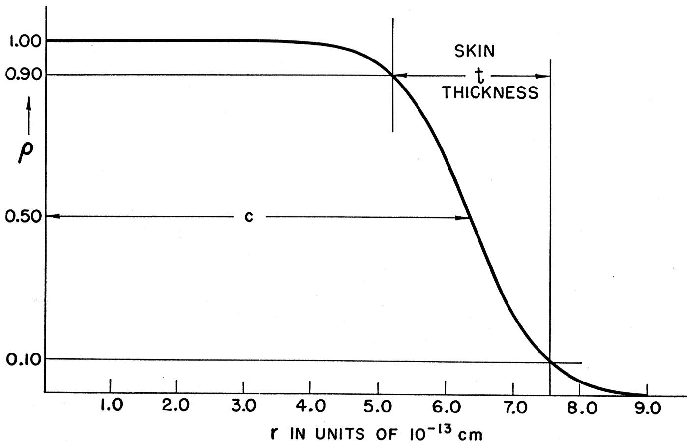
Fig. 8. The shape and parameters which describe an approximate model of the gold nucleus. This type is called the Fermi model (9).
