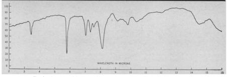
To check composition of lining material in jar lids, a jelly manufacturer uses the IR-5A to identify material as vinyl chloride-acetate copolymer.
