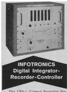
This CRS-1 (Control Recording System) accepts the output signal of any common gas chromatograph and converts it to digital values of both occurrence time and relative area. Accurate digital values of peak times and areas are then recorded simultaneously in any of the common formats: digital printer or typewriter, punched IBM cards, punched paper tape, or magnetic tape using the INFOTRONICS R-1 digital magnetic recorder.
