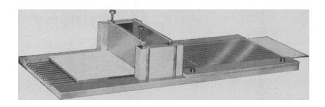
(Thin Layer Chromatography)\* The latest laboratory research tool (by Camag) for the separation and purification of lipids, alkaloids, steroids, etc. Offers: rapid separation (often less than an hour), wide choice of developing reagents, small sample requirements, sharp separations. Mechanically—complete control of layer thickness. Descriptive literature and bibliography available from
