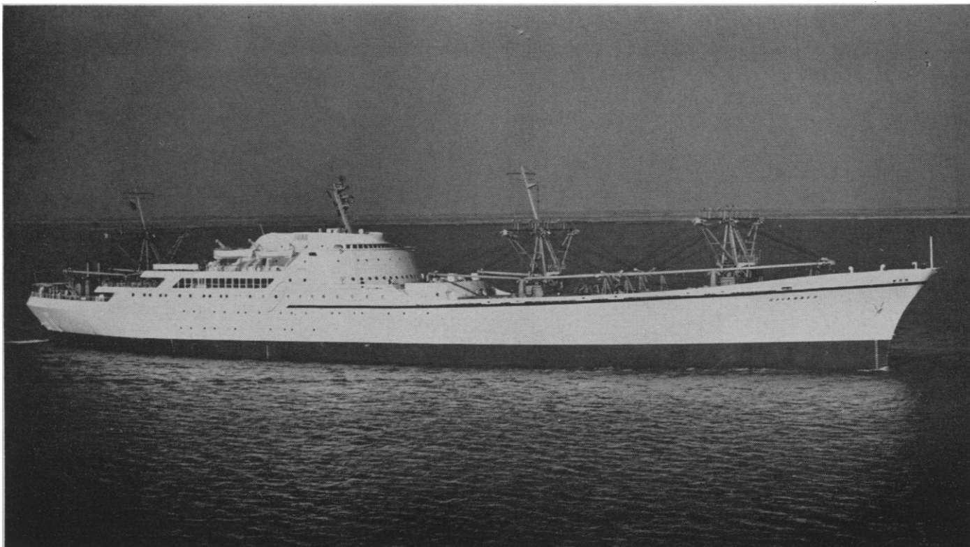
N.S. Savannah , the first nuclear-powered merchant vessel, developed jointly by the Department of Commerce's Maritime Administration and the Atomic Energy Commission. The 22,000-ton vessel, nearly the length of two football fields, is powered by a 69-thermal megawatt pressurized water reactor that produces a normal cruising speed of 20 knots. The reactor holds 17,000 pounds of uranium oxide fuel capable of operating the ship for 3½ years without replacement. Liquid and solid radioactive wastes are collected in monitor-equipped tanks for disposal into a specially designed barge at port; gaseous wastes will be disposed of at sea through the radio mast, equipped with air-particle and radio-gas detectors. The ship will carry 60 passengers, a crew of 110, and 10,000 tons of dry cargo. [Babcock and Wilcox]
