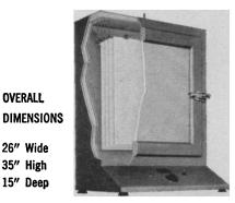
from droplets of combustible solvents. By connecting a motor or water aspirator to the exhaust outlet, heated air is gently circulated over the chromato-grams for fast, uniform drying, as solvent vapors are evacuated.
