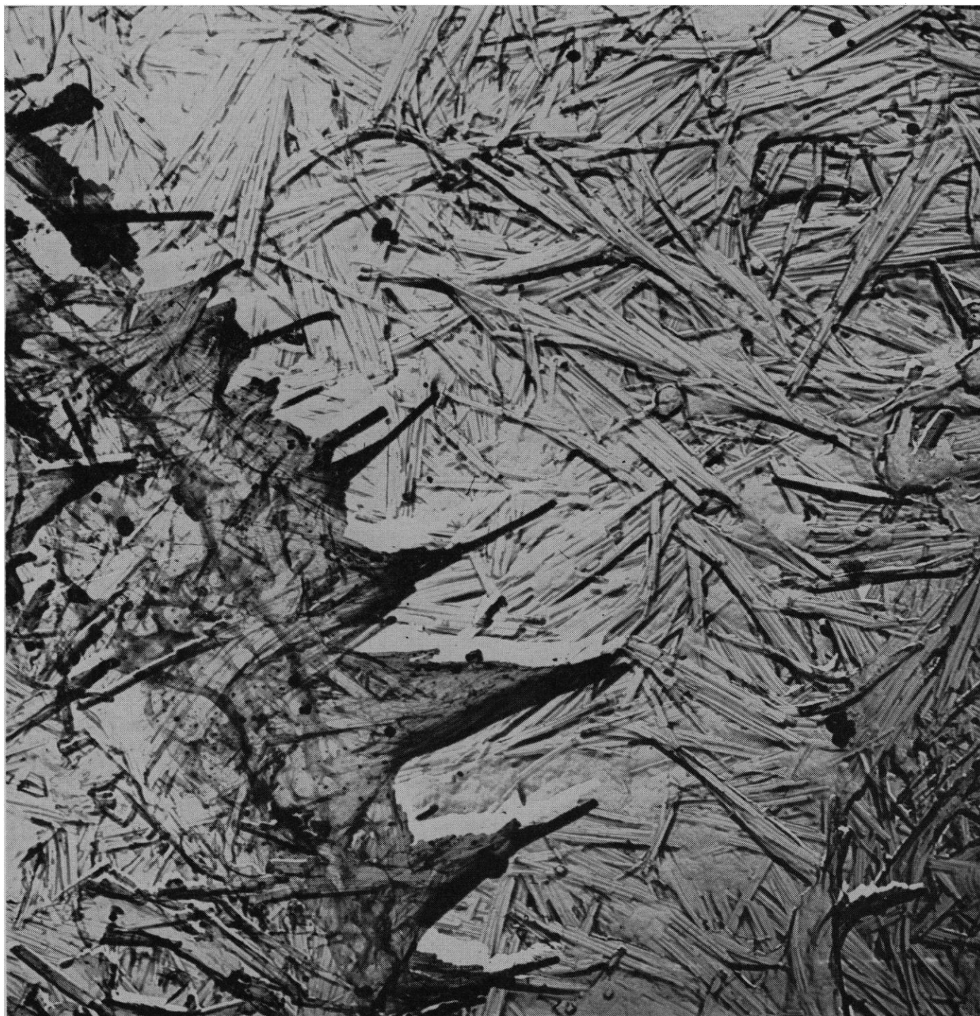
Fig. 7. Electron micrograph of clay composed of fibrous units of attapulgite. (About \times 30,720 ) [From K. M. Towe (7)]
