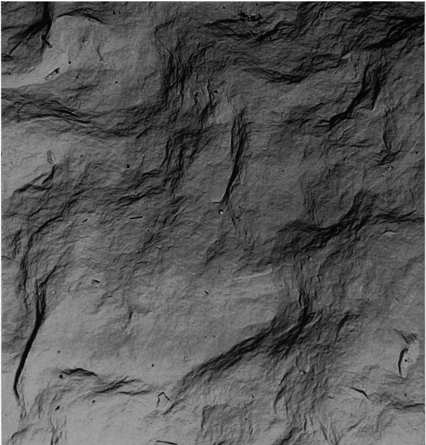
Fig. 6. Electron micrograph of bentonite composed of extremely small units of montmorillonite. (About \times 21,390 ) [From K. M. Towe (7)]
