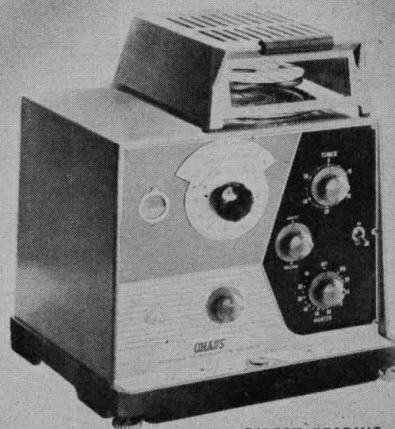
DIRECT READING MOISTURE DETERMINATION BALANCE Capacity 10 Gram Sensitivity .01 Gram—0.1%
