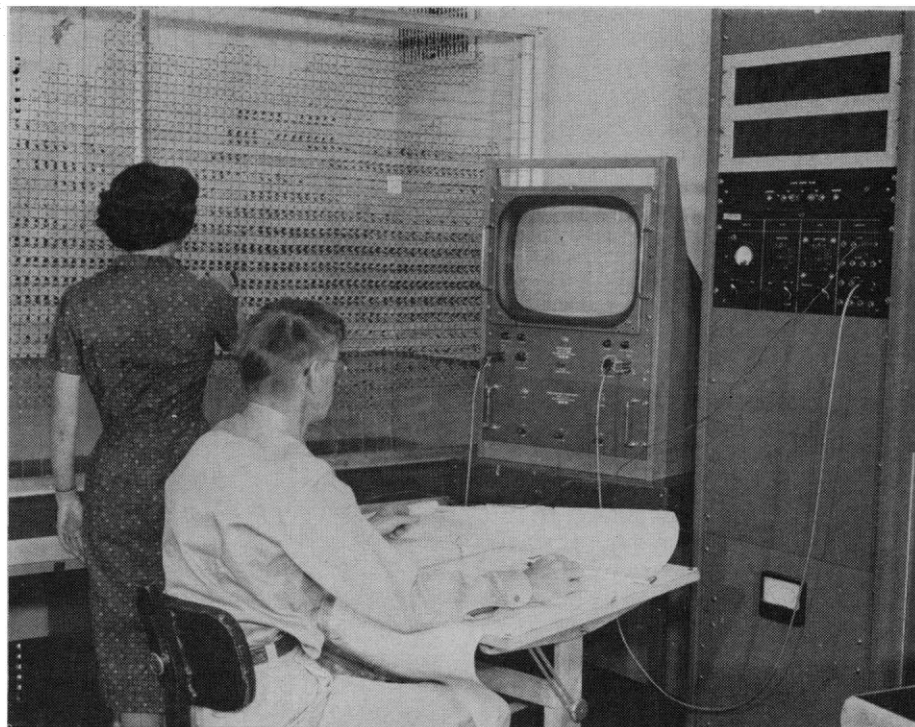
Fig. 2. An analog model of a ground-water aquifer. The analogy between the flow of electricity and the flow of water enables us to use electronic equipment to simulate and therefore solve certain types of hydraulic problems.
