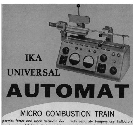
terminations of C, H, N, O, S and Halogens with controlled temperature to 1200°C.
