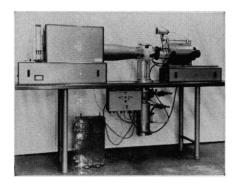
With this instrument dilatation characteristics at temperatures up to 1500°C and in a very high vacuum can be determined.
