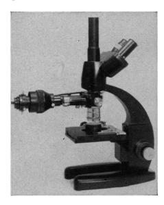
By mounting a substage motion, at little additional cost, the instrument can be used for transmitted light studies in bright field, dark ground, phase contrast and polarized light. Mixed illumination (simultaneous normal incident and transmitted) can be used. In this form, the microscope may be employed on the widest possible variety of specimens.
