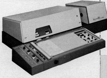
Special applications present no problem to the double-beam, double-monochromator Beckman® IR-4-most versatile of all infrared spectrophotometers. IR-4 design accommodates a wide variety of accessories to meet today's increasing need for unique IR analyses. Instrument down-time for accessory attachment is negligible. And equipping the IR-4 for the *unusual* in no way affects its capability to perform the *usual* qualitative and quantitative studies.
