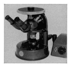
Ball bearing focusing slides, carrying objectives, illuminator and body are of unusual width. These slides subtend the wide angle of 114° at the optical axis — in comparison to a usual value of about 34° in conventional microscopes. This gives the microscope a rigidity which other designs cannot provide.
