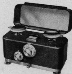
TORSION DWL-2 Capacity: 120 grams Weight-loading Dial: up to 9 grams by 1 gram increments Fine Weighing Dial: 1 gram by .01 gram graduations (Readability: .002 g)
