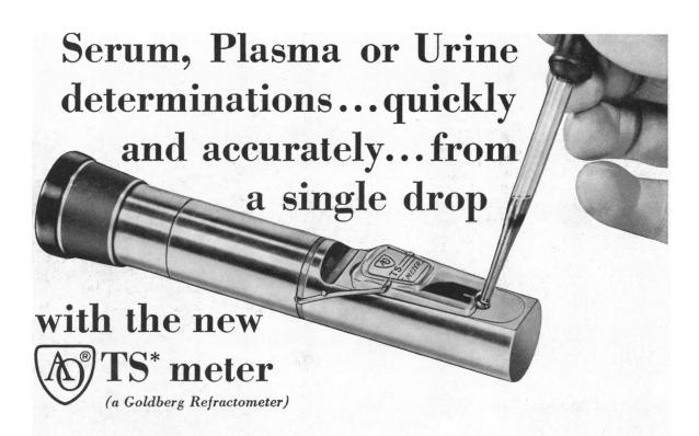
The new AO TS Meter requires just one drop of sample to provide immediate, accurate determinations of total solids, specific gravity, refractive index, protein concentration or water concentration in serum, plasma and urine.
