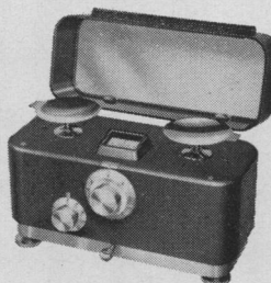
TORSION DWL-2 Capacity: 120 grams Weight-loading Dial: up to 9 grams by 1 gram increments Fine Weighing Dial: 1 gram by .01 gram graduations (Readability: .002 g)
