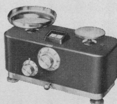
TORSION DWL-5 Capacity: 500 grams Weight-loading Dial: up to 90 grams by 10 gram increments Fine Weighing Dial: 10 grams by .1 gram graduations (Readability: .02 g)
