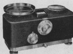
TORSION MODEL DWL-3 Capacity: 200 grams Weight-loading Dial: up to 9 grams by 1 gram increments Fine Weighing Dial: 1 gram by .02 gram graduations (Readability: .005 g)
