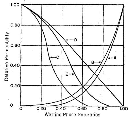
Fig. 1. Relative permeability curves for the network model (curves A, B, C, and D) and for sandstone (curve E). A and C, Wetting and nonwetting phase relative permeability, respectively, based on total volume; B and D, wetting and nonwetting phase relative permeability based on flowing volume; E, nonwetting phase relative permeability for sandstone.
