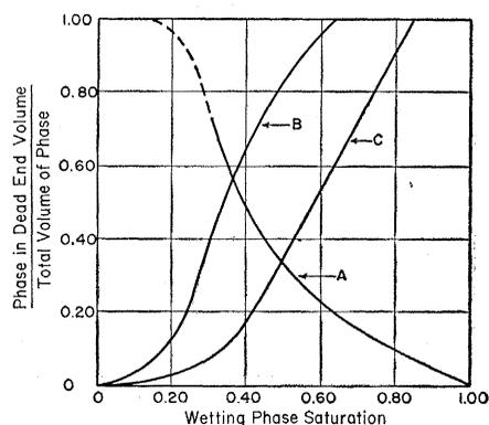
Fig. 2. Fraction of phase trapped in dead-end tubes. A, Wetting phase (from curves A and B of Fig. 1); B, nonwetting phase in network model (from curves C and D of Fig. 1); C, nonwetting phase for sandstone (from curves E and D of Fig. 1).
