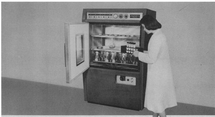
For the Growth of Microorganisms under Controlled Conditions of Temperature, Atmosphere, and Agitation Gassing facilities provided for circulating gas in the tightly sealed chamber.
