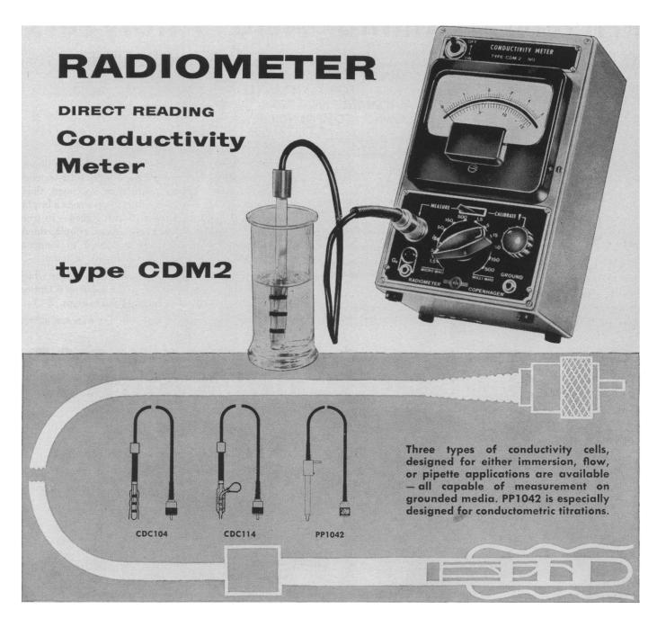
The Radiometer Direct Reading Conductivity Meter fills a long-felt want in any laboratory. Without any sacrifice in accuracy it has been made more flexible and simple in operation than the ordinary conductivity bridge. Direct reading on all of 12 ranges — accuracies better than 1% to 2% are displayed instantaneously on an illuminated and mirrored scale.
