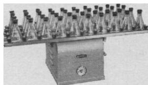
This rugged flat-top unit shakes up to 40 Erlenmeyer flasks or bottles.
