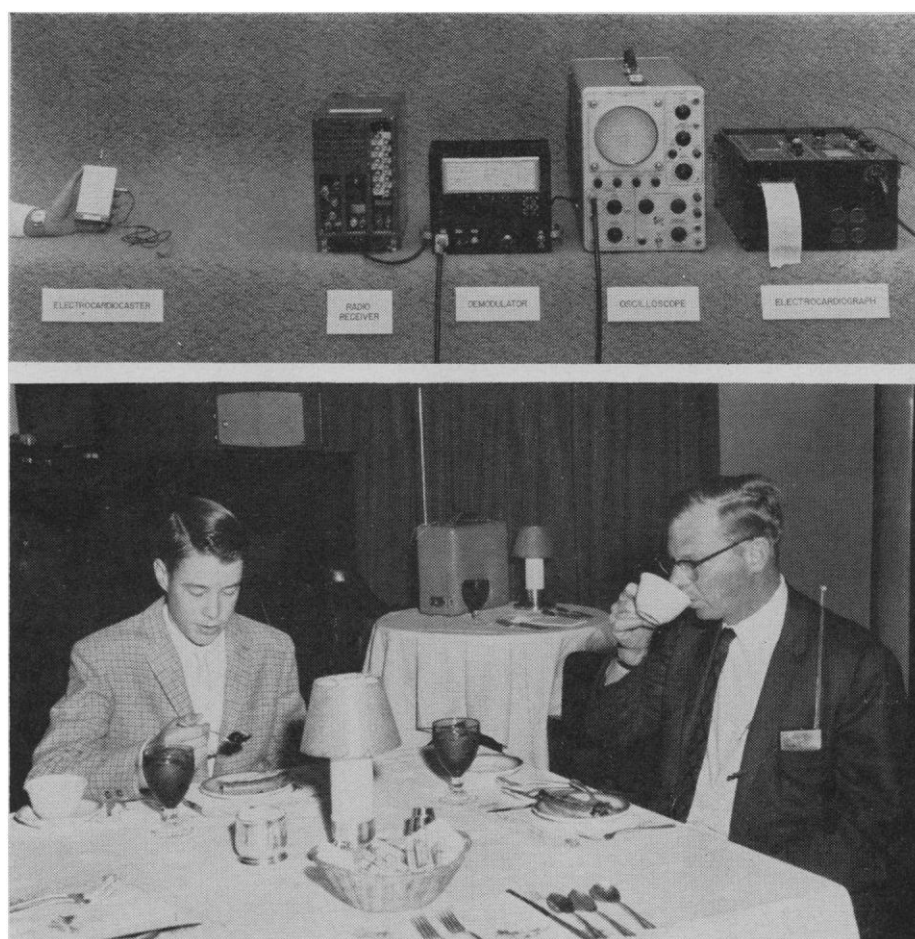
Fig. 1. (Top) Laboratory radioelectrocardiograph system; (bottom) portable version in use.
