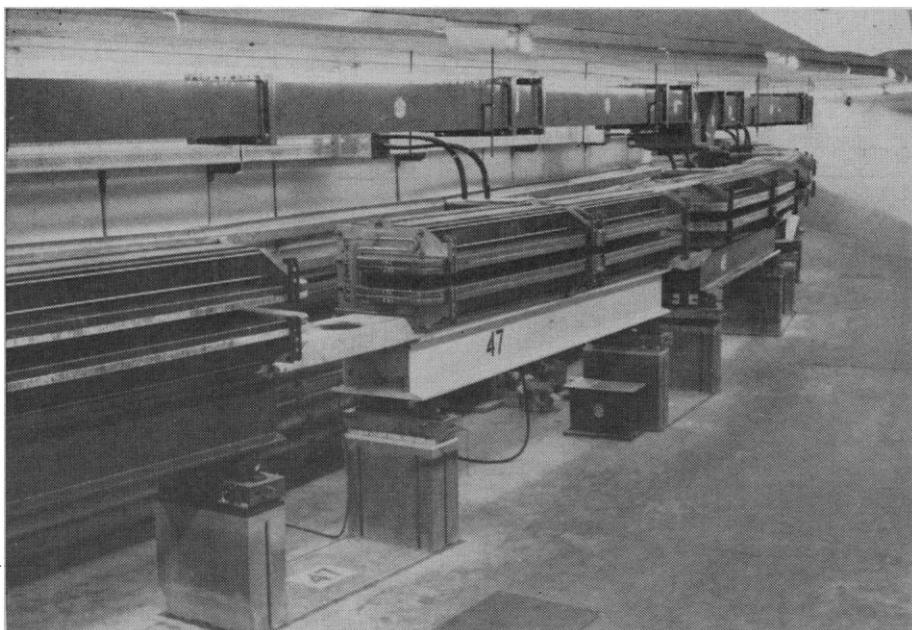
Fig. 2. A portion of the circular array of 48 magnets. Each magnet is 12 feet long and weighs 6 tons. Above the magnets are the radio-frequency waveguides.
