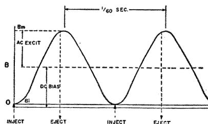
Fig. 4. Wave form of magnetic field strength resulting from the full-biased excitation current. The cycle period is 1/60 second, and nearly half the period is devoted to actual acceleration of electrons.
