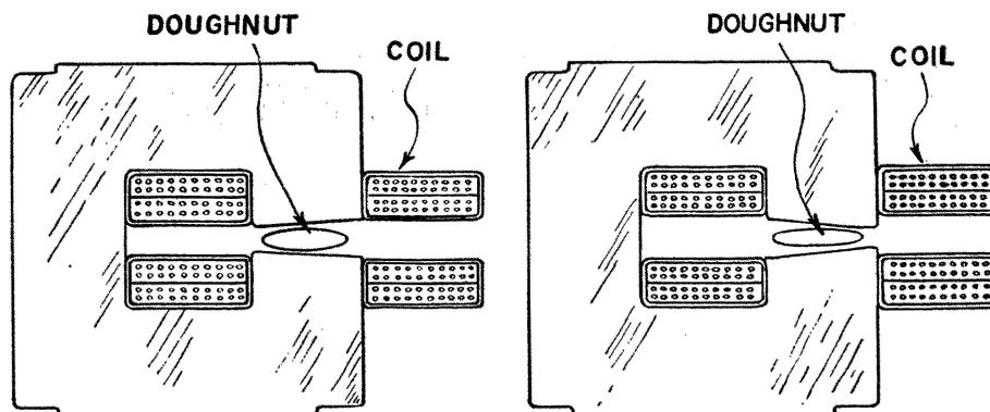
Fig. 3. Cross sections of magnets of (left) the open, vertically-focusing type and (right) the closed, horizontally-focusing type.
