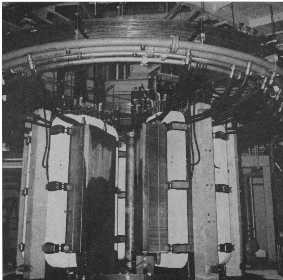
Fig. 8. The 60-ton toroidal inductor for the magnet power supply system (in this photograph one core block and one excitation coil have been removed). The peak energy storage of the inductor is 600,000 joules.
