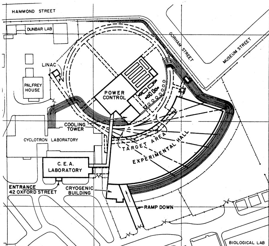
Fig. 1. The general layout of the Cambridge Electron Accelerator. The circular orbit is 236 feet in diameter and is 10 feet below ground level. The experimental hall is as large as a football field.
