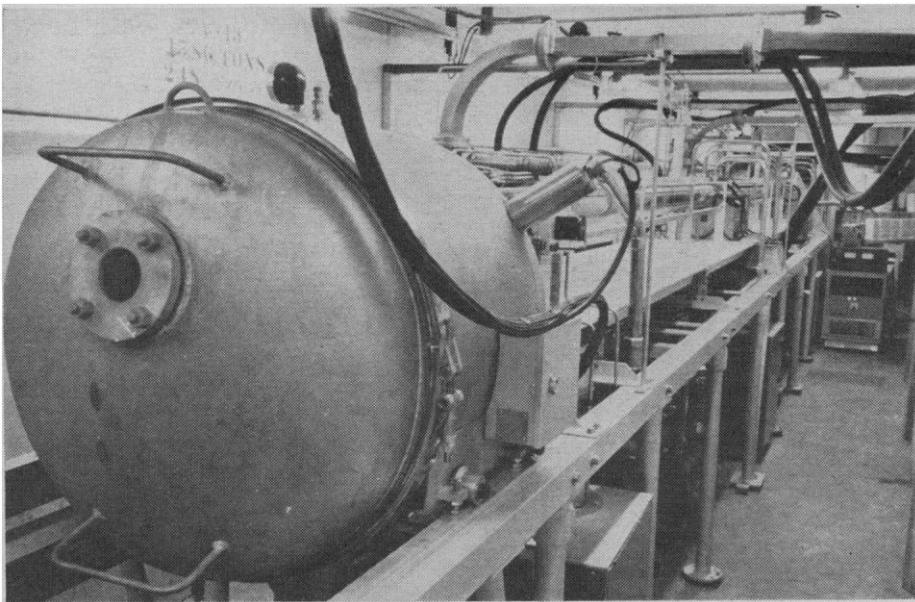
Fig. 5. The 25-Mev linear preaccelerator, which accelerates the electrons from a standing start to a speed of  $0.9998 c$  in a path length of 25 feet. The electrons then enter circular orbit tangentially.
