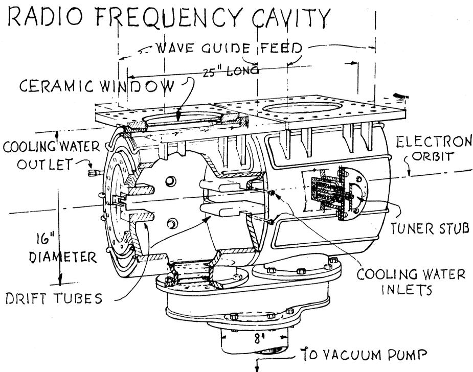
Fig. 6. One of the 16 radio-frequency cavities. The electrons travel along the horizontal axis of the cavity's two resonant chambers and are accelerated by the intense electric fields in the chambers. The fields are supplied by waveguides 18 inches wide (not shown) and air-tight ceramic windows.
