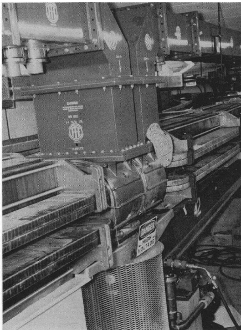
Fig. 7. A radio-frequency cavity in place between two magnets. Above the cavity are the radio-frequency waveguides. Below, suspended from the cavity, is one of the 48 high-vacuum pumps.
