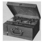
a wide operating range of -10.1 to +100.1 mv and an accuracy of  $\pm (0.05\%)$  of reading  $+3\mu v$  without reference junction compensation;  $\pm (0.05\%)$  of reading  $+6\mu v$  with ref. jct. comp. Write for Data Sheet E-33(1a).
