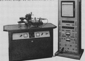
Crystalloflex IV and Electronic Circuit Panel with Diffractometer and Guinier Camera mounted on the generator. SCIENCE, VOL. 134
