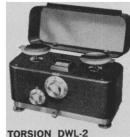
Capacity: 120 grams Weight-loading Dial: up to 9 grams by 1 gram increments Fine Weighing Dial: 1 gram by .01 gram graduations (Readability: .002 g)
