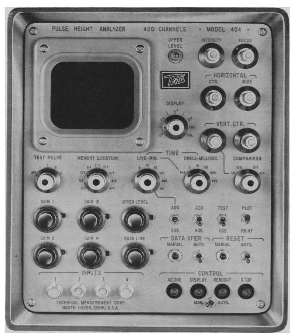
efficient 4-input, 400-channel pulse height analyzer is easy to use, has many "system" features, weighs 37 lbs., occupies one cubic foot, operates on 110 or 220 volts, 50 to 400 cycles AC.
