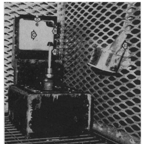
Fig. 1. Apparatus as seen by the monkey (A, control stick; B, meter; C, needle; D, target zone; E, food dispenser).
