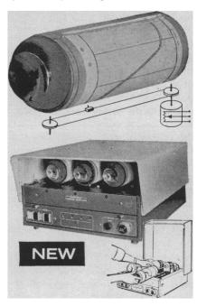
Now, with only an ordinary graphite pencil and graph paper, you can feed program instructions to automatic process controls. Data-Trak follows pencil-drawn graphs anyone can prepare. High degrees of accuracy and reliability result from use of unique capacitive curve-following principle. Potentiometer output is proportional to drawn curve.
