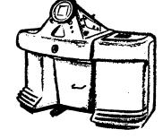
tures like the Norelco *immersion lens* which alone makes possible many unusual techniques such as free manipulation and even deformation of the specimen while under observation.
