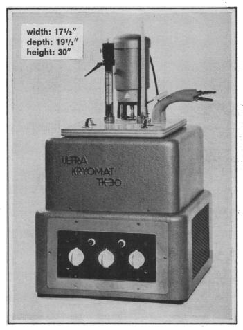
Introducing the world's first table model Kryomats for low temperature control—offered in two models. Range from +20 to -30°C.
