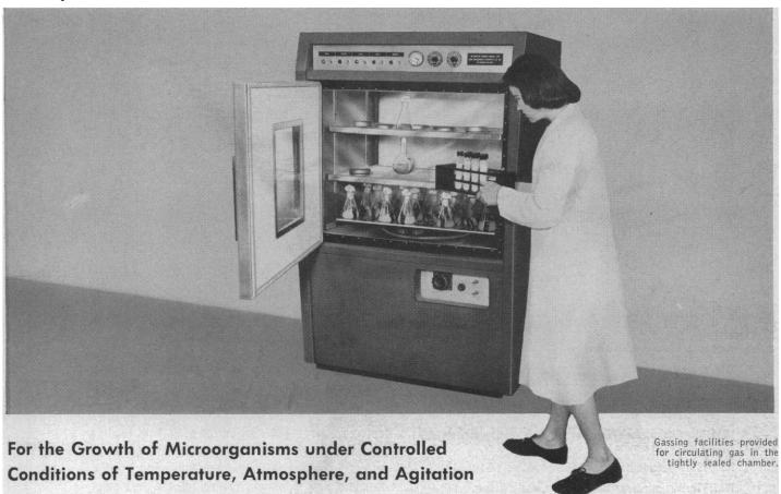
THE PSYCROTHERM is a rigidly controlled environmental incubator with a continuous-duty shaking mechanism. Though it occupies comparatively little floor area, it has 10½ cubic feet of *usable* work space in the incubation chamber, where static and shake cultures can be incubated simultaneously or separately.
