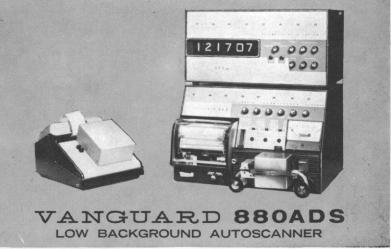
Data obtained with the ADS, representing actual counts within a given zone of the chromatogram, is processed by the ADS logic circuitry and printed in numerical form. Entire zone activity, incremental sub-zone areas, and entire strip activity may be presented individually or in various combinations. No other system provides the accuracy, speed and dynamic versatility of the Vanguard Model 880ADS.
