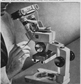
SNAP shutter with cable release. You photograph the sharp three-dimensional image exactly as you saw it. Your film processor will supply stereo mounted photographs. Now you have permanent, three-dimensional photomicrographs, in black-and-white or color, for future reference.
