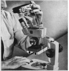
SWING the mounted 35mm Graflex Stereocamera into position over eyepieces. Designed exclusively for Cycloptic, special compensating prisms in adapter unit render camera parfocal with microscopes' optical system. Set camera for bulb exposure. No further adjustment is necessary.
