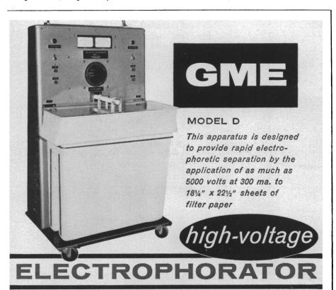
In order to dissipate the heat thus generated, the paper is immersed in a bifurcated fiberglass tank containing Varsol, which is a light petroleum fraction. It has a high flash point (over 100 degrees C.), does not conduct electricity, and has the proper degree of volatility for this application. The Varsol is cooled by stainless steel coils at the top of the tank. Cold tap water is adequate as a coolant.
