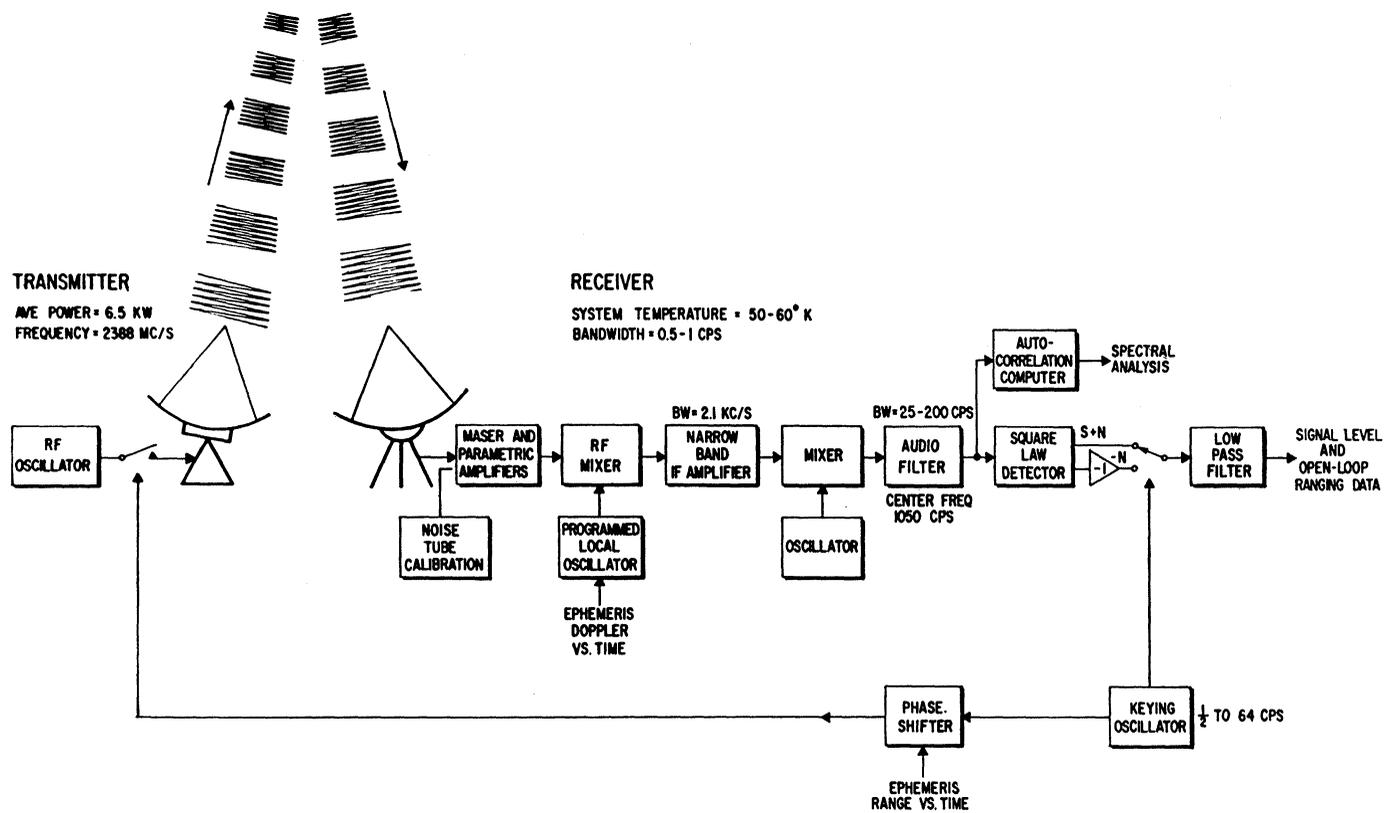
Fig. 1. Venus radar with nonsynchronous open-loop receiver.
