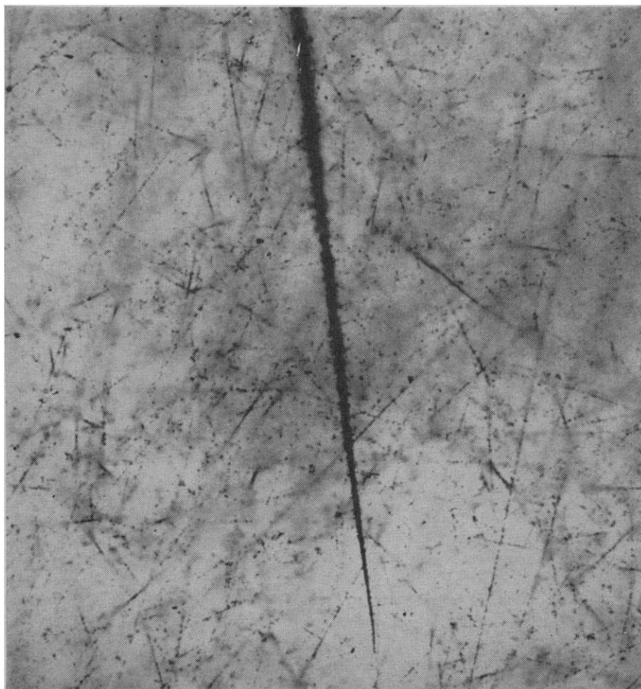
A typical photomicrograph of tracks obtained during the time Discoverer XVIII's re-entry capsule was in orbit. [Cambridge Research Laboratories, U.S. Air Force]
