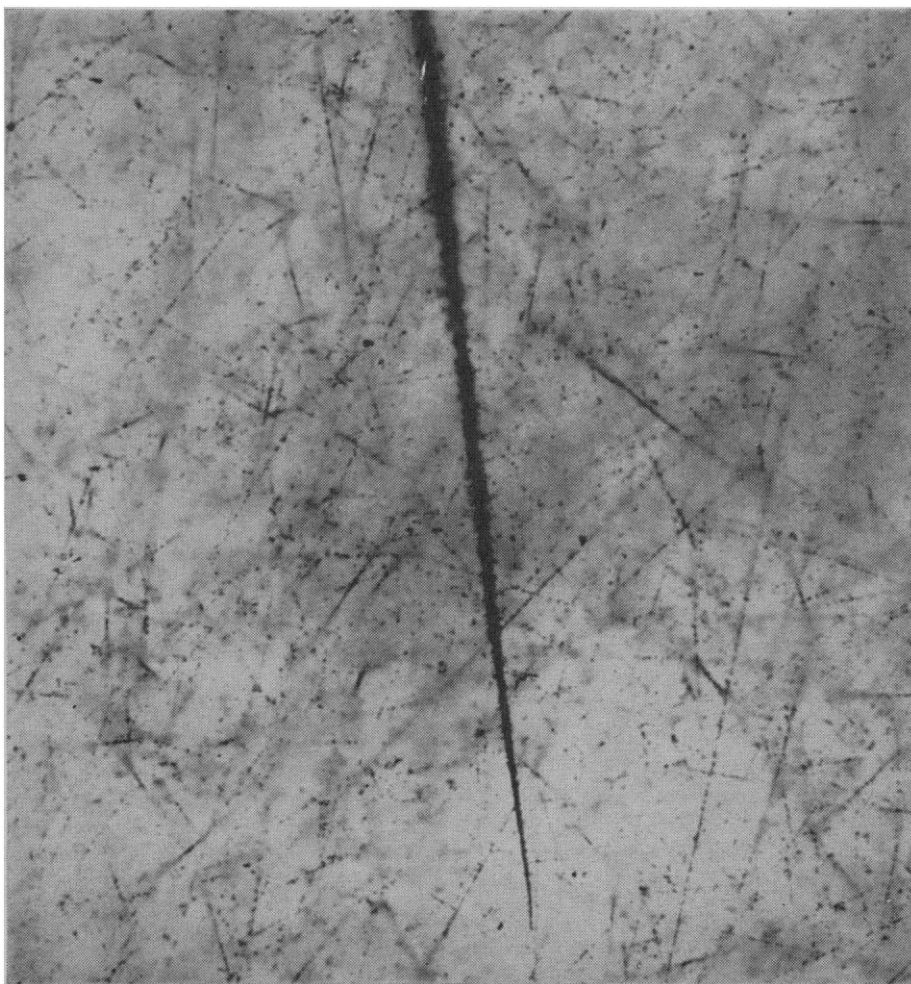
A typical photomicrograph of tracks obtained during the time Discoverer XVIII's re-entry capsule was in orbit. [Cambridge Research Laboratories, U.S. Air Force]
