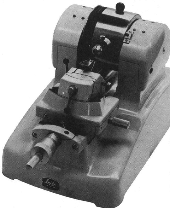
Microtome mounts on specially designed table for vibration-free rotor drive. Control panel housed in convenient safety-lock drawer. Stereoscopic microscope and lamp are mounted on a carrier arm of microtome with lateral swing-out movement. Draft-free microtome cover prevents air circulation from disturbing specimen while sections are being cut.
