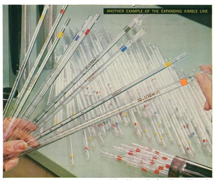
Each size of KIMAX serological pipets (#37034 and #37034-A for cotton plugging) is coded with its own identifying color band.
