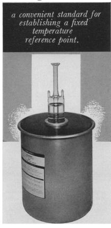
EQUIPHASE Triple-Point-of-Water Cell establishes a reference temperature of 0.01°C with guaranteed accuracy of 0.0005°C. Unaffected by atmospheric pressure, contamination-free, easy and convenient to use. Just 17" high, 8" diameter.
