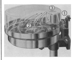
Stokes Automatic Laboratory Water Stills produce distilled water that's completely free of bacteria, pyrogens, and minerals. They give you distillate that contains less than 2 parts per million impurities . purer than the standards set by United States and British Pharmacopoeia.
